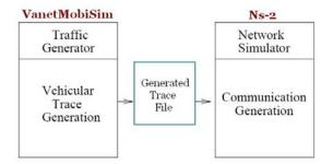
Figure 1: Simulator basic architecture.
